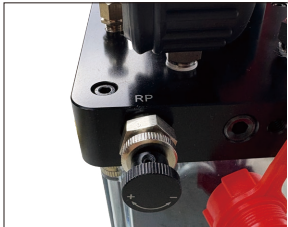
Rotate the pressure regulating valve slowly in a clockwise ('+') direction.
