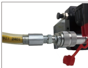
Turn the outer lock ring tight
