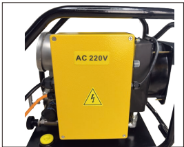
Check the electronic control box to determine the rated voltage.
