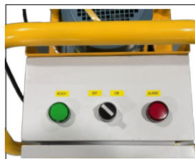
Connect the power supply. The "READY" green light ON the left side will light up. Turn the rotary switch to the "ON" position and start under pressure.
