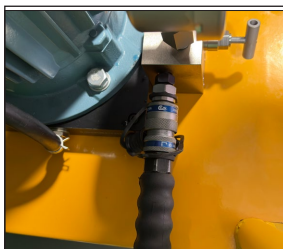
The outer lock ring is pushed back, and the oil pipe is fully pushed into the outlet by axial alignment.
