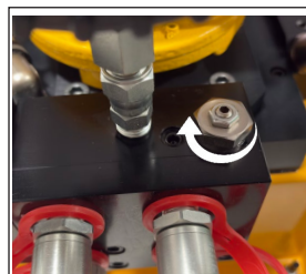
The return pressure is regulated by the R-port pressure limiting valve.
