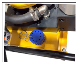
If the oil level is lower than 2/3, please rotate and remove the plug of this outlet, and then carry out the refueling operation.
