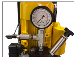
In the no-load state of the system, confirm that the initial reading of the pressure gauge is zero.
