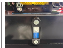
Hydraulic oil level gauge
