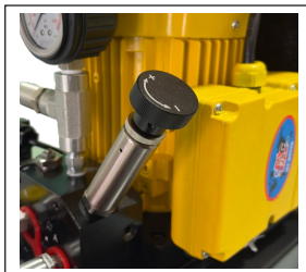
Loosen the locking nut on the relief valve and rotate the relief pressure regulating valve clockwise slowly to achieve the target pressure at port A.
