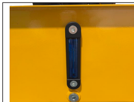
Hydraulic oil level gauge
