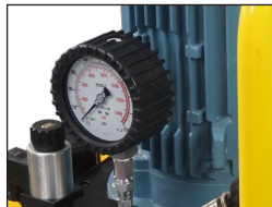
When the system is unloaded, the pressure gauge displays the pressure at port R.
