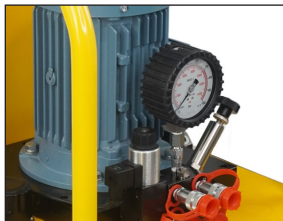
Through the electromagnetic valve control button on the handle, the oil flow direction of the system can be accurately controlled.
