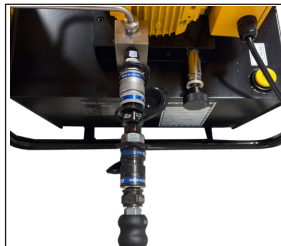
After pushing the oil pipe, push the outer lock ring forward and rotate it clockwise to lock.
