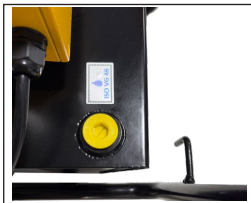
If the oil level is lower than 2/3 of the upper oil gauge scale line,the outlet plug should be removed and the hydraulic oil replenishment operation should be performed.
